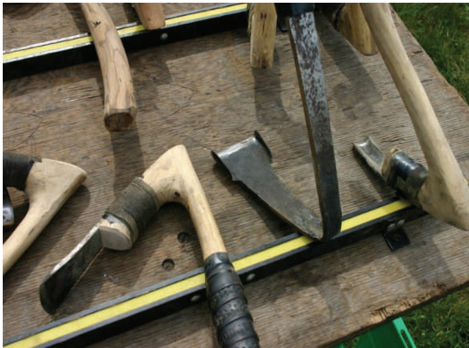
Forging a slick (a large chisel looking tool used like a wood plane) from a truck leaf spring
