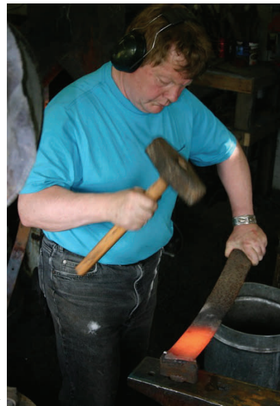
Forging a slick (a large chisel looking tool used like a wood plane) from a truck leaf spring
