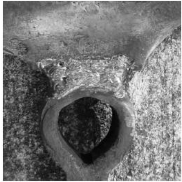
Figure 4: Anvil welded to post.
