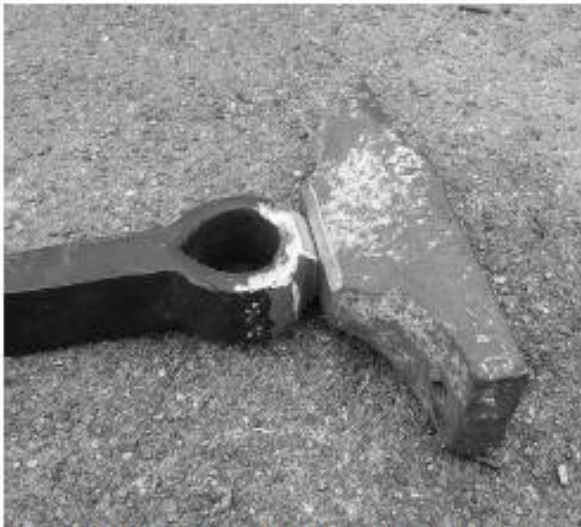
Figure 2: Dry-fit anvil and leg showing the ground bevels
