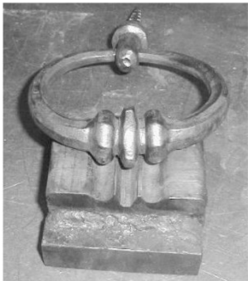
Examples of power hammer swages (courtesy of David Ponsler)
