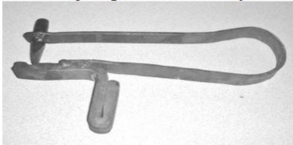
Groover for putting the lines in the candy cane ↓
