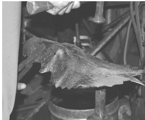
2. Pattern is cut from 1/8" steel then textured. He made a triceratops head for the demo.
