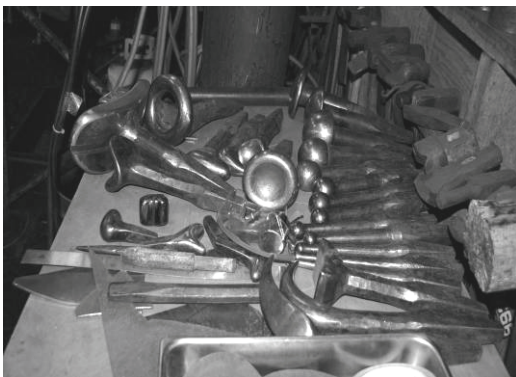
5. Some of the stakes he has made to form the steel
