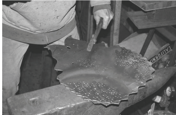
2. Pattern is cut from 1/8" steel then textured. He made a triceratops head for the demo.
