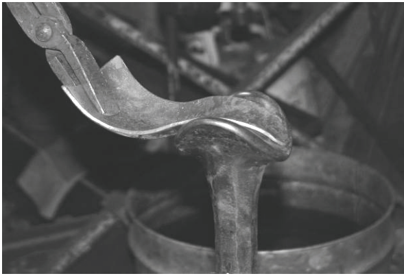
7. Making a horn using a saddle shaped stake
