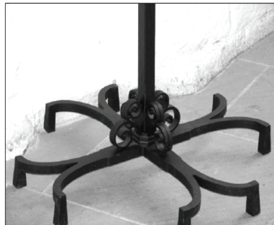
The feet are split, then bent, from the same 2" (5.08cm) stock.
