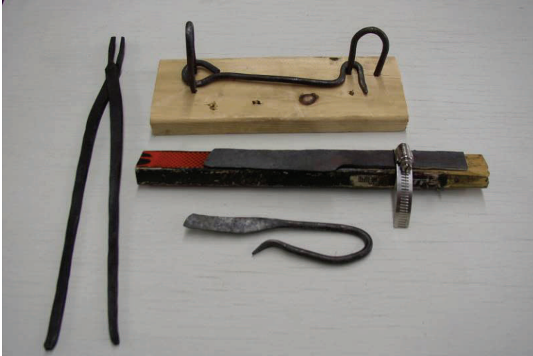
Gate Latch, Starter tongs, and knife clamp from hockey stick and hose clamp from Don Startin
