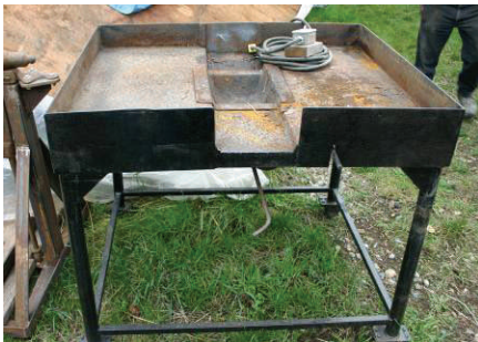
Used coal forge and firepot with electric blower
